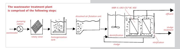
Industrial wastewater treatment plants often have to treat very complex wastewater to an extend that allows for subsequent use of the treated water as process water or for discharging it to the sewer.
