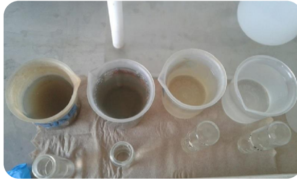
Figure 1. From left to right: raw influent, DAF effluent, MBR permeate and tertiary effluent.
