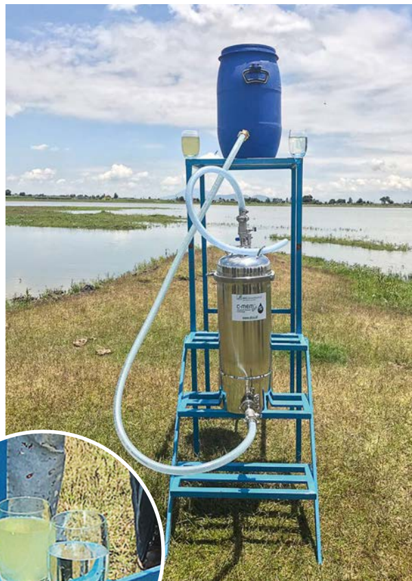
Filtration test at Toluca Lagoon / Mexico; raw water vs. clear water after filtration
