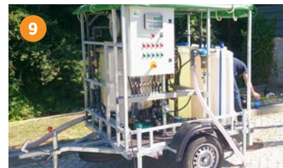
9 Angola/Africa mobile treatment unit drinking water (source: surface water) 100 m 3 /d
