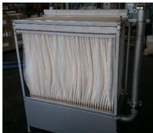
The biological treatment takes place in the MBR tank. Due to the membrane, all biomass in the form of activated sludge is held back and therefore, the sludge age can be freely chosen. Aeration on the bottom of the tank ensures aerobic degradation of organic substances, as well as prevents sludge particles from clogging the membrane.
