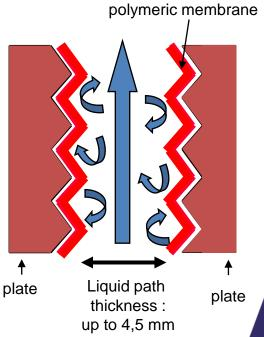
Open channel (means no spacer)
