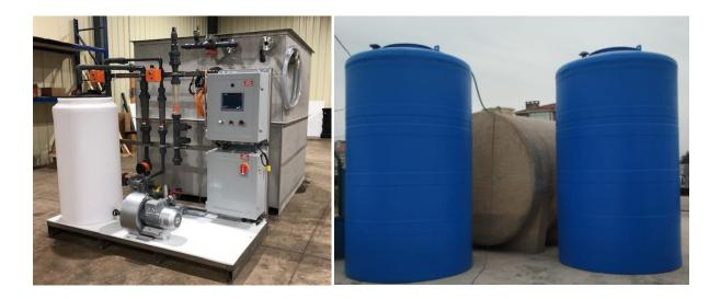
Once on-site, the Prefabricated Membrane Filtration Module (316SS) & BioReactor Tanks (FRP) were plumbed together easily with pre-identified tie points.
