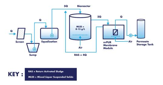
The activated sludge process converts the soluble organic material present in the wastewater into  $CO_2$ ,  $H_2O$  and biological cell mass. An aeration system provides the oxygen required for this process. The mass of oxygen transferred is based upon the design daily influent BOD load.
